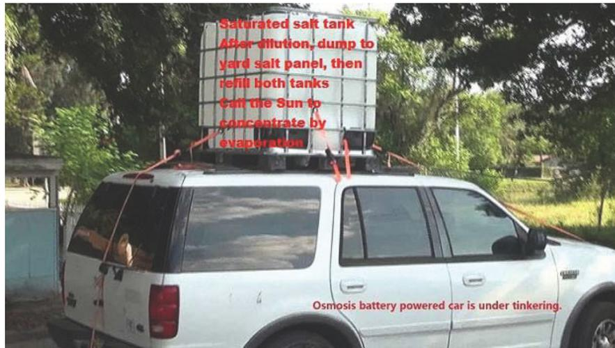
Above prototype is heavily dependent on home-base evaporation pool or solar distillation recharging backend. After exhausted, both water tank and saltwater tank of the vehicle must be refilled and replaced respectively.
